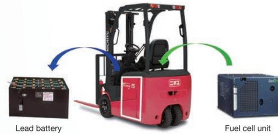
Fig. 1 Replacement with a fuel cell unit
