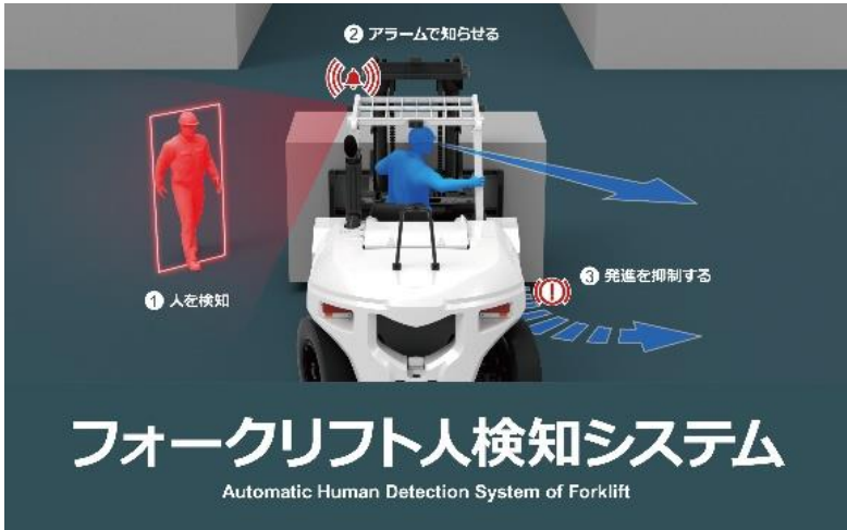
Automatic Human Detection system of Forklift
